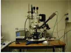
In vivo scanning tonometry setup: thin glass pipette (tip diameter 10-80 μm) delivers the air flow to the sample, the spot of light reflected by the surface of the sample is detected by the camera, attached to the microscope
