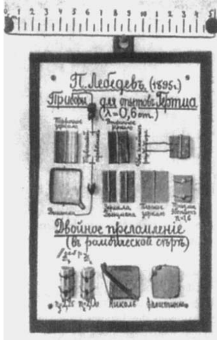
Figure 15.6. The components designed by P. Lebedev for his Hertz-type experiments at the wavelength \lambda = 6 mm in 1895 (reproduced from [31]).
