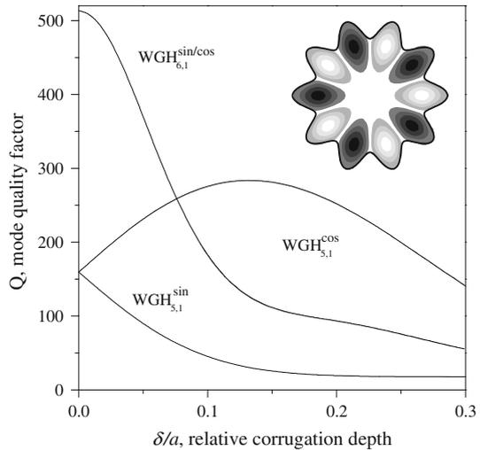
**Fig. 5** Q-factors of the deformation-matched and mismatched ( $H_z$ ) $_{5,1}$  modes in a GaAs notched circular cavity as a function of the notch depth normalised to the cavity radius;  $\alpha_{\text{eff}} = 2.64$ ,  $\lambda = 1.55 \mu\text{m}$
