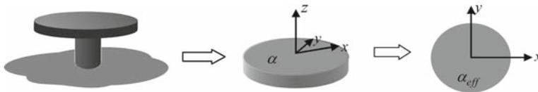
**Fig. 1** Reduction of the layered disk-on-pedestal electromagnetic problem to the homogeneous 3-D free-space disk and to the 2-D circular-cavity model based on the effective refractive index concept
