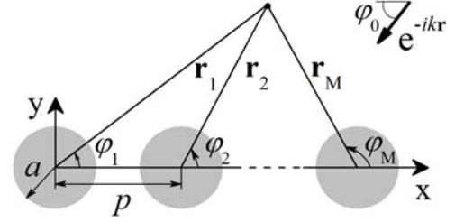
Fig. 1 Cross-section of the linear grating of circular wires under the plane wave incidence
