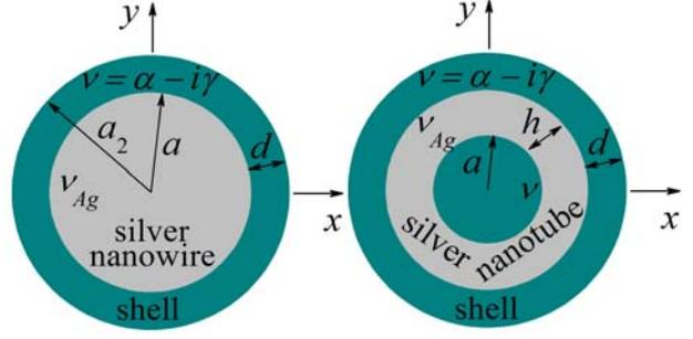
Fig. 10 Cross-sections of nanolasers based on silver nanowire and nanotube
