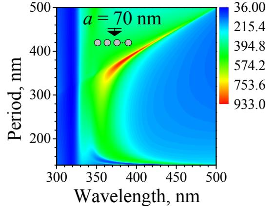
Fig. 3 Relief of TSCS as a function of the wavelength and the period for a linear grating of 100 silver nanowires
