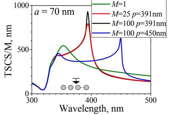
Fig. 2 TSCS as a function of the wavelength for linear gratings of silver nanowires
