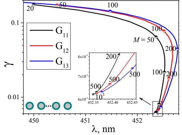
Fig. 14 Trajectories of the LEP eigenvalues of modes  $G_{11}$ ,  $G_{12}$  and  $G_{13}$  on the plane  $(\lambda, \gamma)$  for the gratings of Fig. 13 if the wires number  $M$  varies
