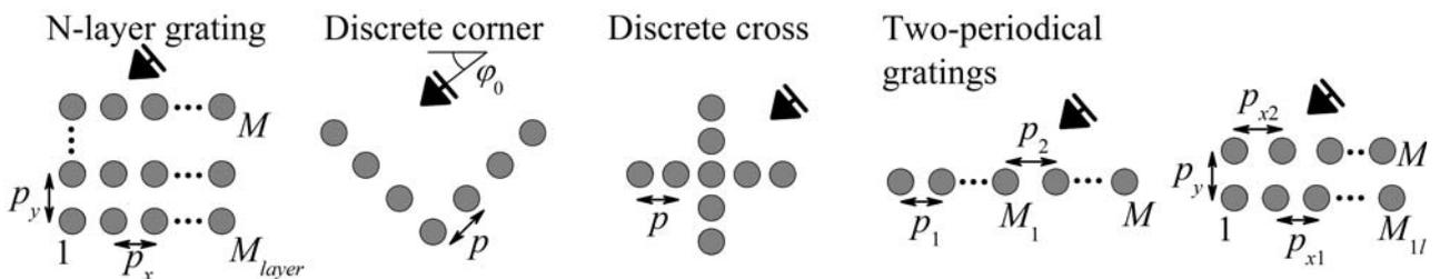
Fig. 5 Cross-sectional views of the grating configurations considered in Ch. 3
