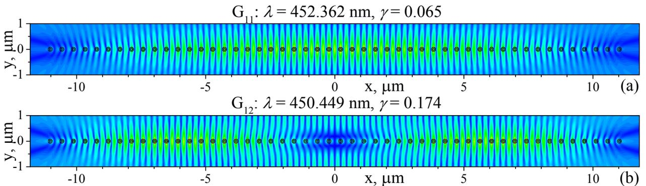
Fig. 13 Near fields of the grating modes  $G_{11}$  and  $G_{12}$  of the grating of 50 silver nanowires with the core radius  $a = 40$  nm and active shells with  $\alpha = 1.414$  and the thickness  $d = 40$  nm, collected in the grating with period  $p = 450$  nm
