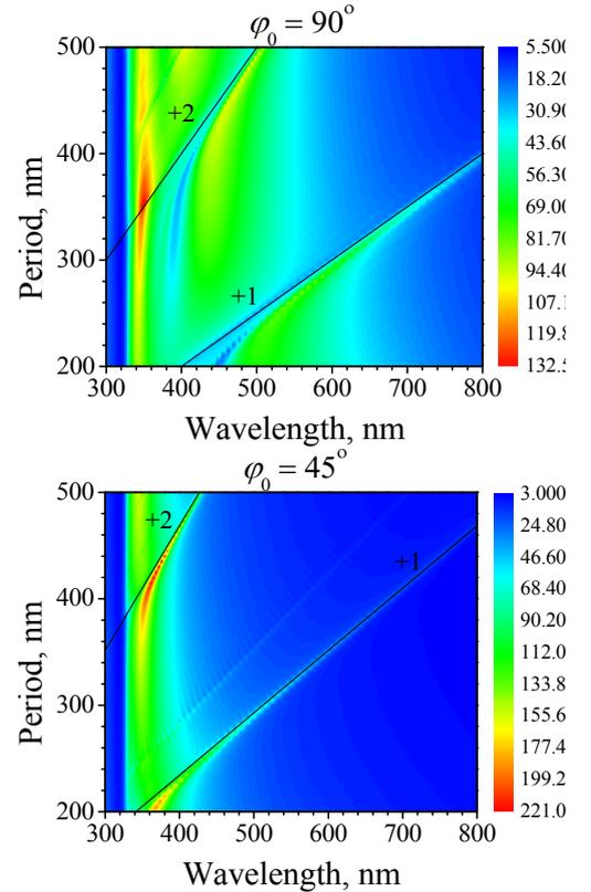
Fig. 6 Color maps of TSCS as a function of the wavelength and the period for a discrete cross of 101 silver nanowires with the radius of 30 nm
