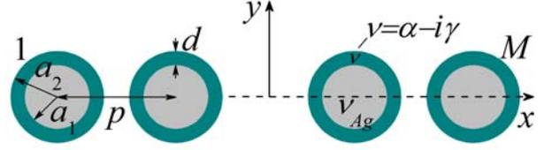
Fig. 12 Cross-section of the grating of  $M$  silver nanowires with active shells
