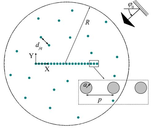
Fig. 8 Cross-section of the grating of silver nanowires inside a cloud of the same wires
