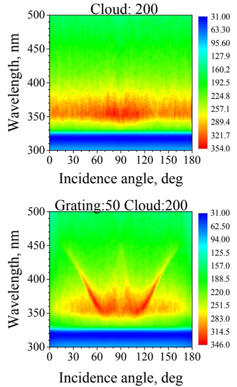
Fig. 9 Color maps of TSCS as a function of the wavelength and the incidence angle for a cloud of 200 silver nanowires and for the same cloud with the grating of 50 nanowires placed approximately in the cloud center
