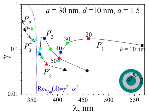
Fig. 11 Trajectories of the eigenvalues of silver nanotube laser modes under a variation of its thickness (in nm)
