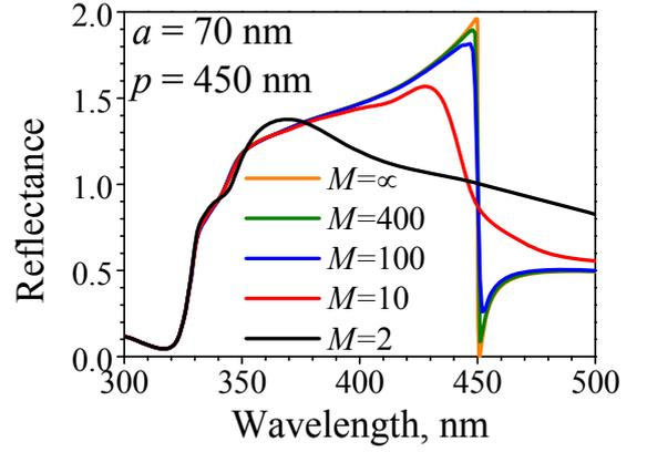
Fig. 4 Normalized reflectance as a function of the wavelength for finite and infinite gratings of silver nanowires
