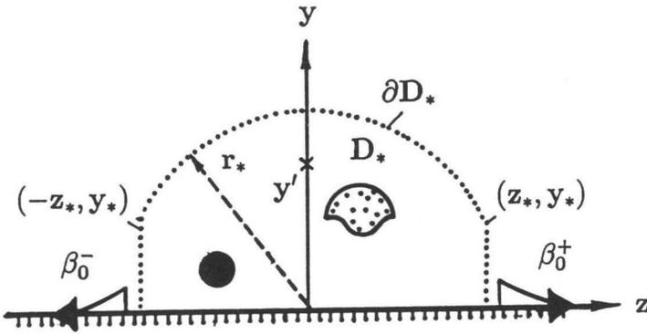
Figure 1. Two-dimensional geometry of localized scatterers near an impedance plane.
