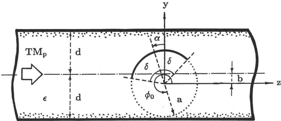
**Figure 5.** A particular 2-D geometry for a circular screen inside a dielectric slab. One of the natural guided modes is incident.
