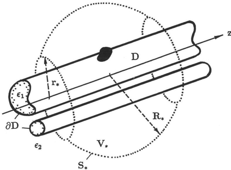
Figure 4. Three-dimensional geometry for a dielectric core open-waveguide scattering.
