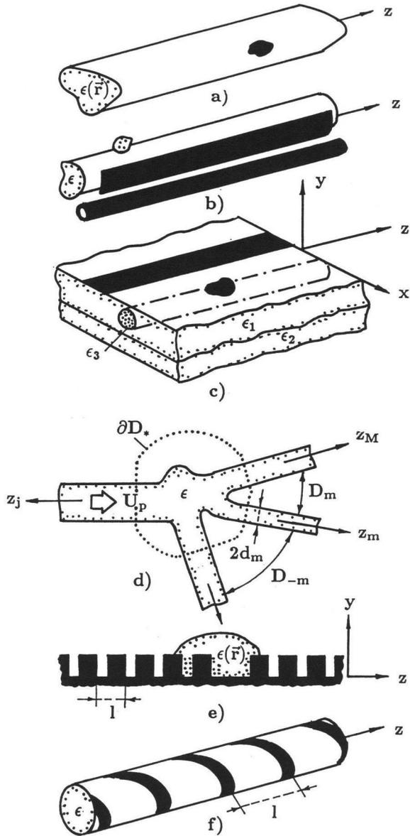
**Figure 7.** Examples of more complicated open waveguides containing localized inhomogeneities
