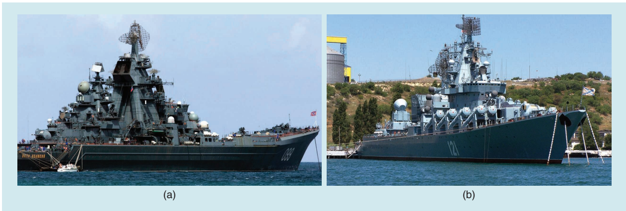
FIGURE 8. (a) “Legenda” satellite receiver antennas on the Pyotr Velikiy nuclear-powered USSR cruiser (a)—white radome on a vertical structure at the side of the tower—and (b) on the sunken Moskva cruiser (b)—similar light-grey radome just above the rear launch tube. To eliminate the shadowing of antennas, the same equipment was placed at the portside.
