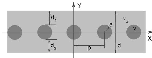
Fig. 1 Cross-sectional geometry of a periodically perforated dielectric slab
