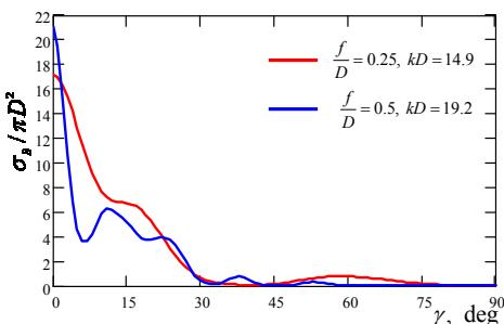
Fig.5. Paraboloidal reflector  $f/D = 0.5$  and  $f/D = 0.25$  normalized backscattering cross section as a function of the angle  $\gamma$ .
