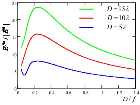
Fig. 9. The electric field module in the paraboloid geometric focus as a function of  $f/D$  in the case of  $D=5\lambda, 10\lambda, 15\lambda, \gamma=0$
