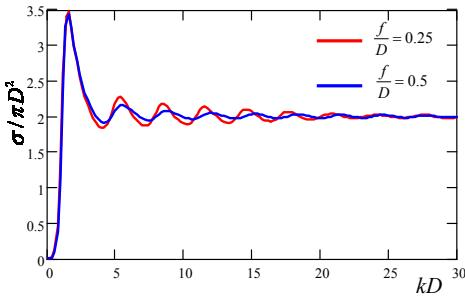
Fig.4 Paraboloidal reflector  $f/D = 0.5$  and  $f/D = 0.25$  normalized total scattering cross section in the case of the orthogonal incidence ( $\gamma = 0$ ).
