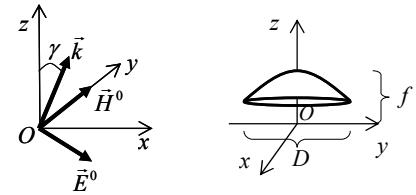
Fig. 2 Parabolic reflector illuminated by the electromagnetic plane wave
