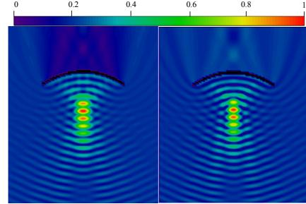
Fig. 7. The near fields of the paraboloidal reflector  $f/D = 0.5$  illuminated by the plane wave in  $kD = 19.2$  in the E-plane (left) and the H-plane (right)
