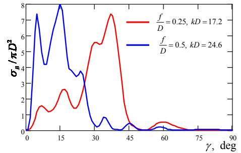
Fig.6 Paraboloidal reflector  $f/D = 0.5$  and  $f/D = 0.25$  normalized backscattering cross section as a function of the angle  $\gamma$
