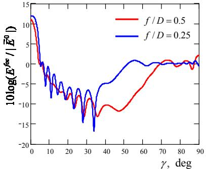
Fig. 11. The electric field module in the paraboloid geometric focus as a function of the angle  $\gamma$  in the case of  $f/D = 0.25, 0.5, D = 10\lambda$ .
