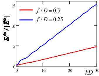
Fig. 10. The electric field module in the paraboloid geometric focus as a function of normalized frequency in the case of  $f/D = 0.25, 0.5, \gamma = 0$ .
