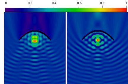
Fig. 8. The near fields of the paraboloidal reflector  $f/D = 0.25$  illuminated by the plane wave in  $kD = 14.9$  in the E-plane (left) and the H-plane (right)
