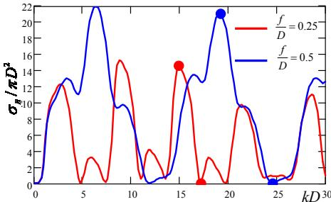
Fig.3 Paraboloidal reflector  $f/D = 0.5$  and  $f/D = 0.25$  normalized backscattering cross section in the case of the orthogonal incidence ( $\gamma = 0$ ).
