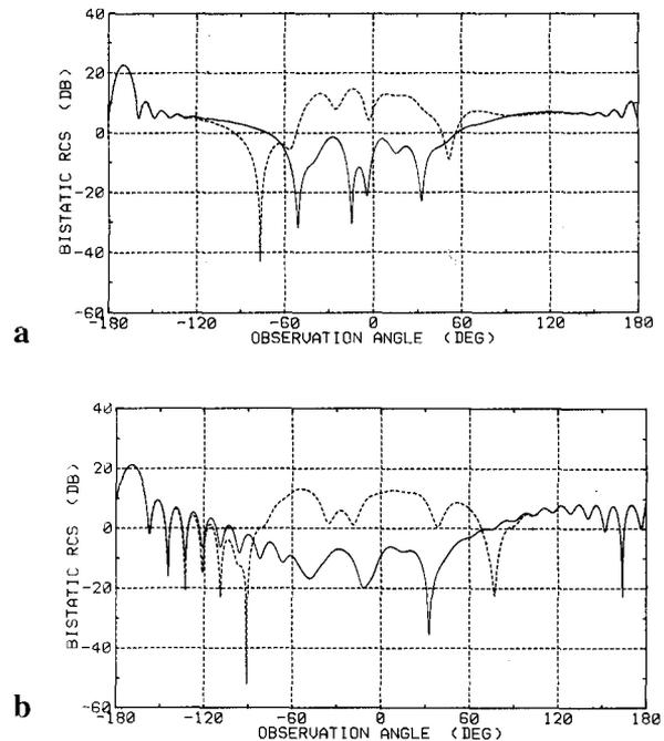
FIG. 8. — Bistatic RCS (dB) versus observation angle  $\phi$  of a circular cavity with  $\phi_0 = 10^\circ$ ,  $ka = 15.7$ ,  $\theta = 45^\circ$ ,  $t/a = 0.1$  ( $t = d - c$ ).
