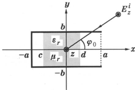
FIG. 1. — Geometry of the rectangular cavity.
