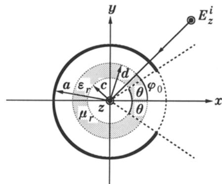
FIG. 2. — Geometry of the circular cavity.
