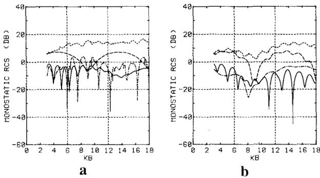
FIG. 3. — Monostatic RCS (dB) versus normalized frequency  $kb$  of a rectangular cavity with  $\varphi_0 = 10^\circ$ ,  $a/b = 1.0$ ,  $t/a = 0.2$  ( $t = d - c$ ).
