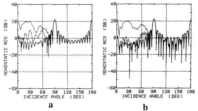
FIG. 5. — Monostatic RCS (dB) versus incidence angle  $\varphi_0$  of a rectangular cavity with  $kb = 15.7$ ,  $a/b = 1.0$ ,  $t/a = 0.2$  ( $t = d - c$ ).
