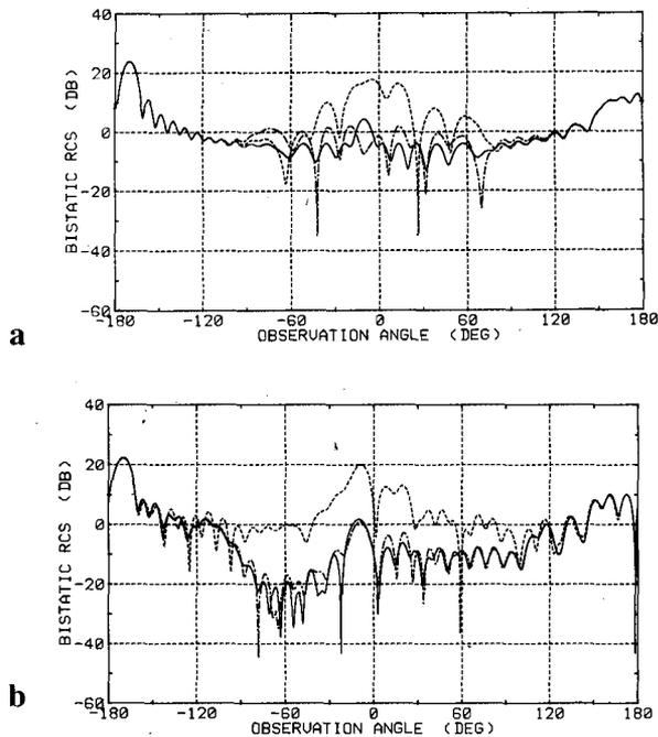
FIG. 7. — Bistatic RCS (dB) versus observation angle  $\phi$  of a rectangular cavity with  $\phi_0 = 10^\circ$ ,  $kb = 15.7$ ,  $a/b = 1.0$ ,  $t/a = 0.2$  ( $t = d - c$ ).
