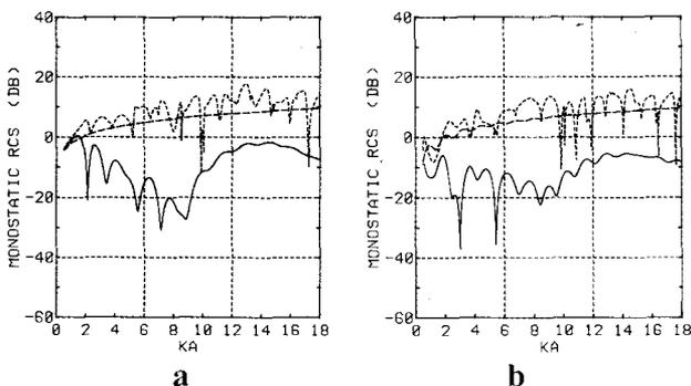
FIG. 4. — Monostatic RCS (dB) versus normalized frequency  $ka$  of a circular cavity with  $\varphi_0 = 10^\circ$ ,  $\theta = 45^\circ$ ,  $t/a = 0.1$  ( $t = d - c$ ).
