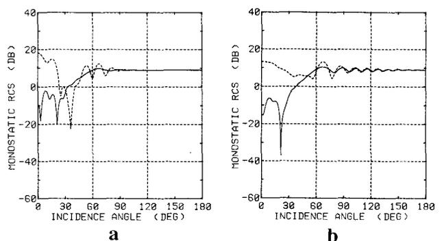
FIG. 6. — Monostatic RCS (dB) versus incidence angle  $\varphi_0$  of a circular cavity with  $ka = 15.7$ ,  $\theta = 45^\circ$ ,  $t/a = 0.1$  ( $t = d - c$ ).
